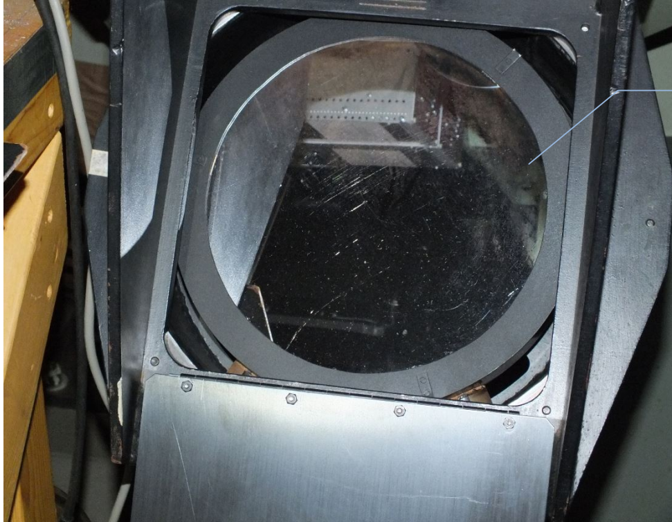
Collimator mirror with fragile coating and degradation at top and right side
