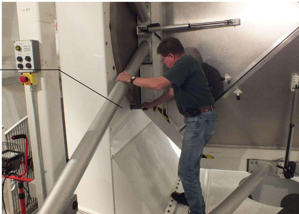
Pinning the telescope in horizontal position
