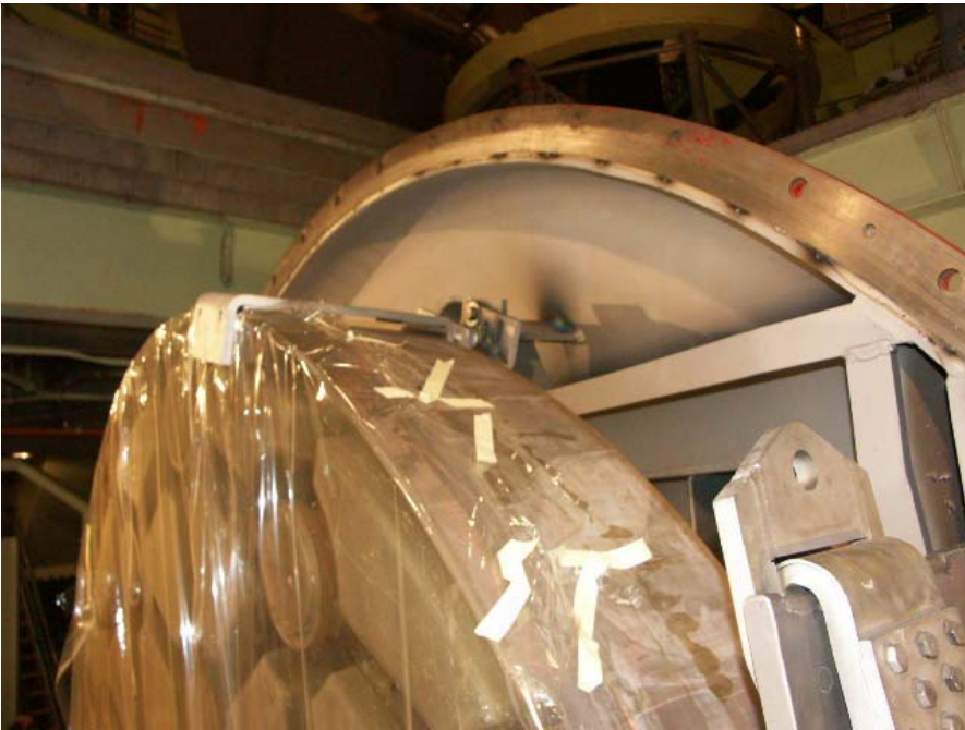
The mirror was anchored from moving inside the tank by a custom connection between the "earthquake clamp" on the mirror at the top.
