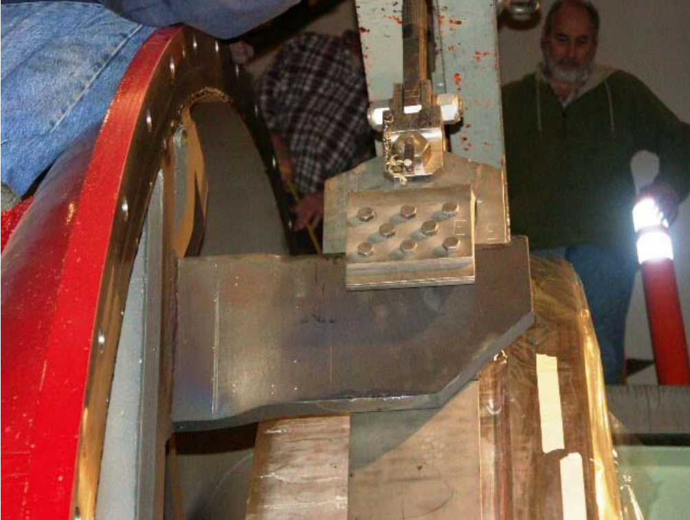
The mirror was anchored from moving inside the tank by a custom connection between the "earthquake clamp" on the mirror at the top.
