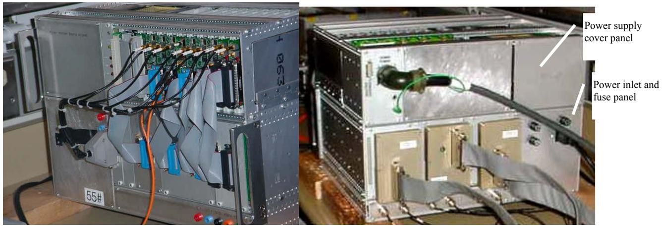
**Figure 17: CCD controller**
