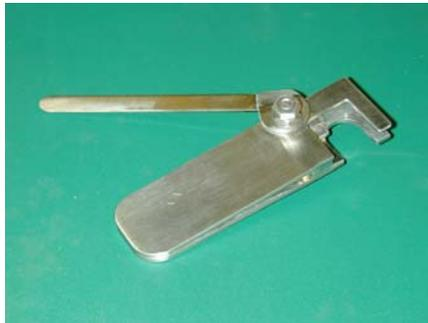
Figure 15: Analog Switch Board Extractor
