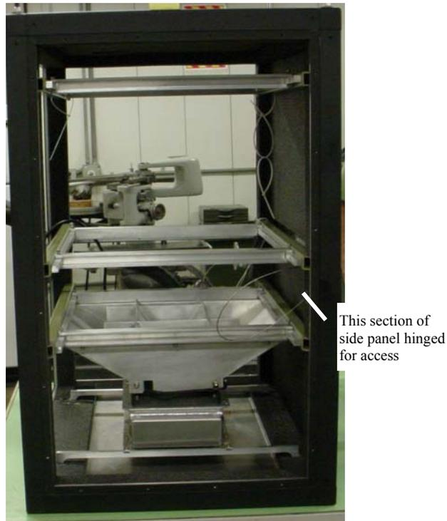
**Figure 20: Footlocker without electronics or front and rear cover panels**
