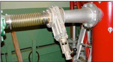
Open the valve located between the Roots blower and cold trap. (left)
