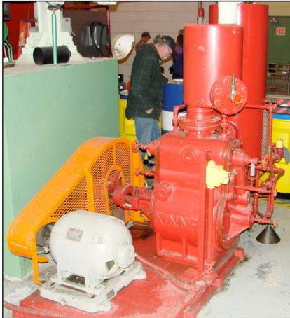
Next turn on the Kinney pump (yellow switch housing) and start pumping on the back side of the diffusion pumps.
