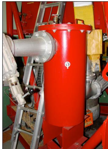
Climb the ladder enough to remove the cover from the trap and fill the center hole of the trap with the dry ice. Use the stick that is located by the trap to tamp the ice periodically to keep the ice in good contact with the sides of the trap.
