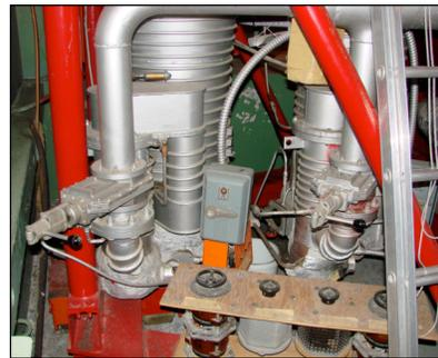
Open the two DP booster valves located to the left of the cold trap. That will help keep the pumps cool while waiting to open the DP main valves.
