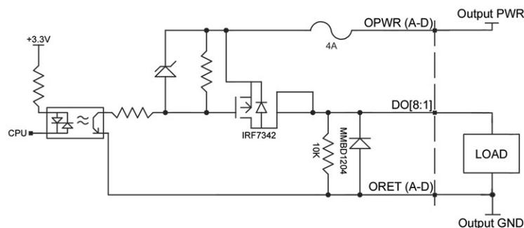
Figure 3.6: 500mA Sourcing wiring diagrams for Bank 0, DO[8:1]
