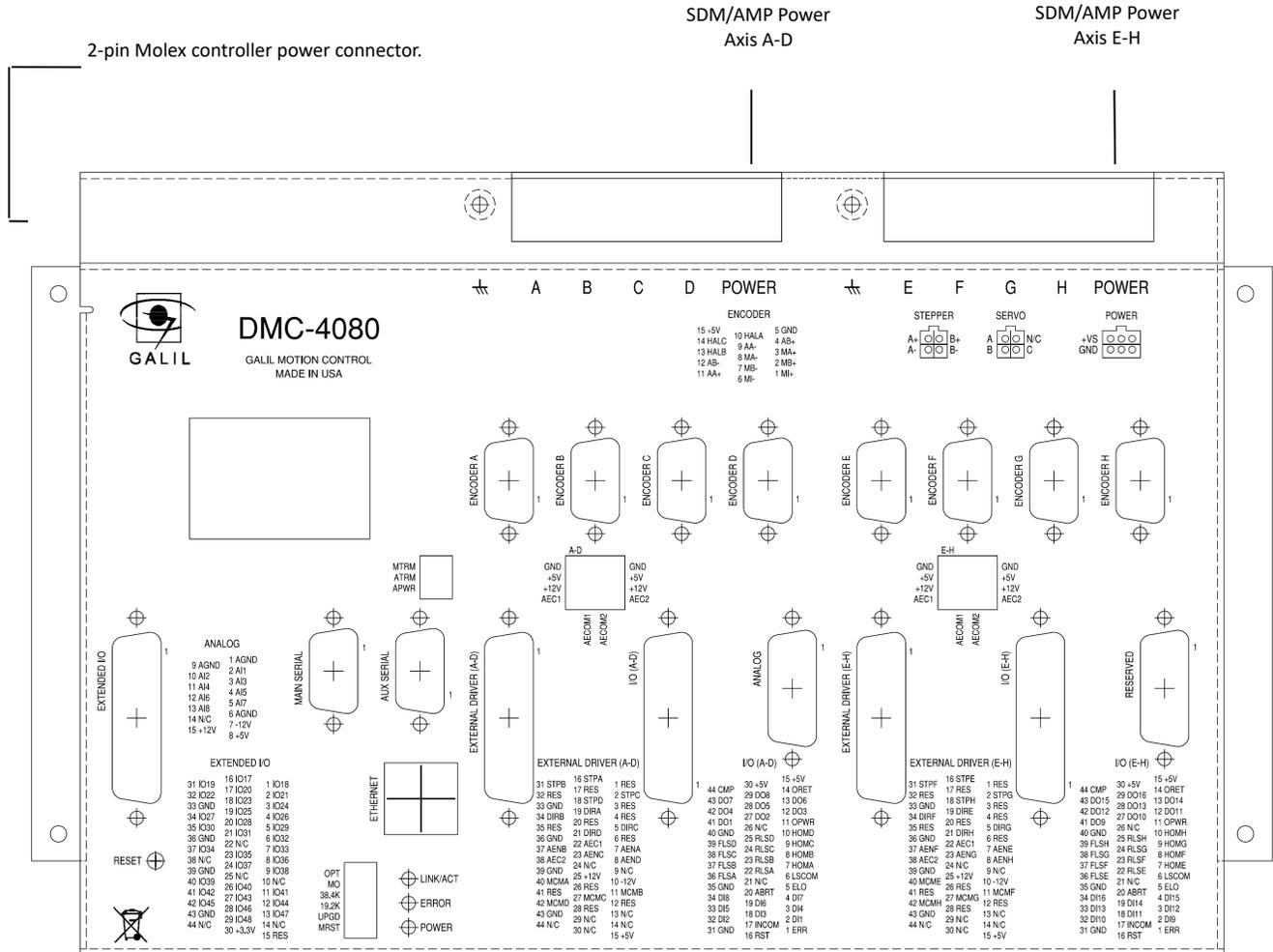
Figure 2.3: Power Connector locations for the DMC-40x0
