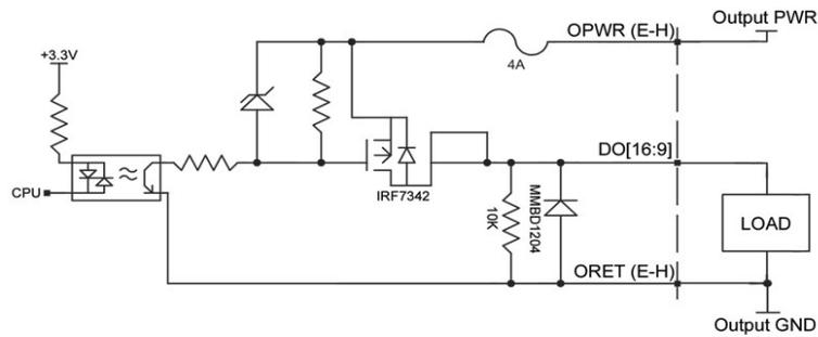
Figure 3.7: 500mA Sourcing wiring diagram for Bank 1, DO[16:9]
