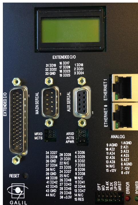
The CMB-41022 differs from the CMB-41012 (default) in that it has second Ethernet port, as shown in the figure above. The CMB provides the connections for both Ethernet and Serial communication as well as the 44-pin HD D-Sub connector for the Extended I/O. An 8x2 character LCD screen is used to display the status of each axis, or can display a custom message if desired.
