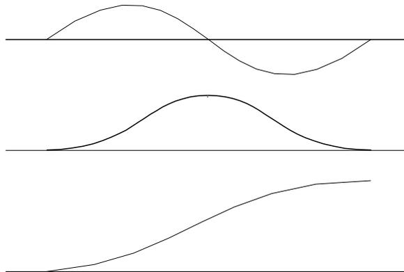
Figure 6.19: Velocity Profile with Sinusoidal Acceleration
