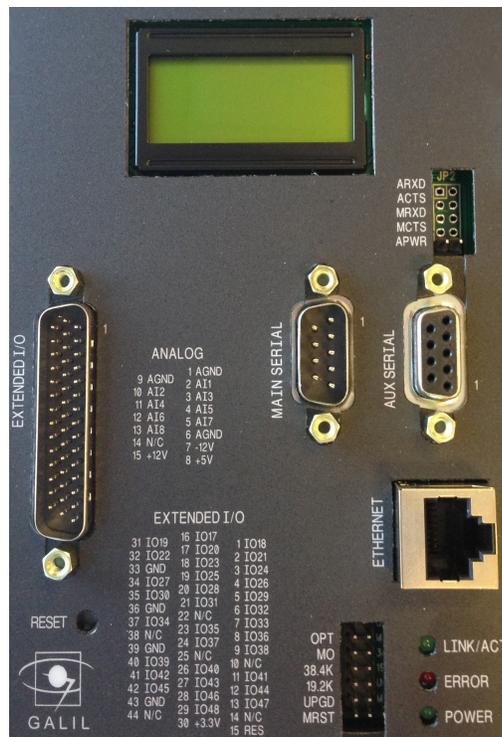
The CMB-41012 provides the connections for the Ethernet and Serial communication as well as the D-Sub connector for the Extended I/O. The CMB-41012 also contains the 8x2 character LCD.
