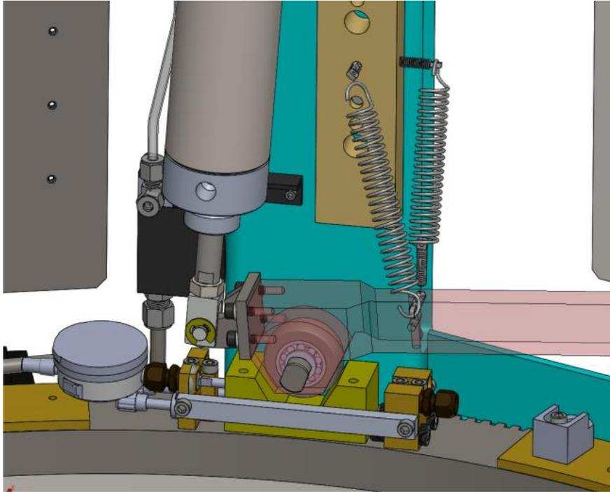
Figure 22: K1DM3 Instrument Position Detent Adjustment Mechanism
