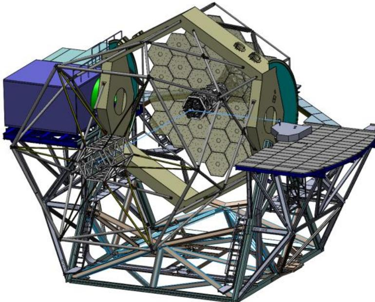
Figure 19: Setup of secondary socket mounted alignment telescope on Keck 1, blue highlighted line represents center ray from alignment telescope to K1DM3 to AO system mounted auto-collimation mirror
