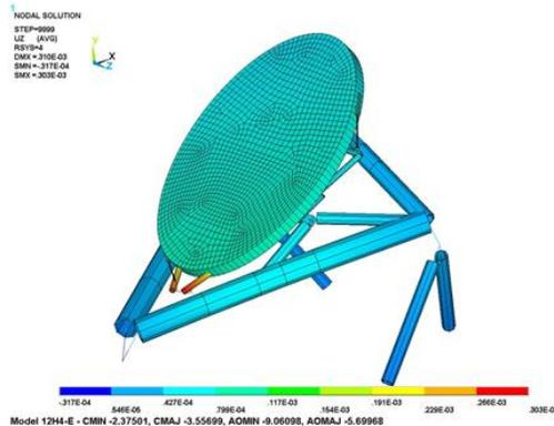
Figure 10 - FEA model of the combined swing arm and mirror assembly.
