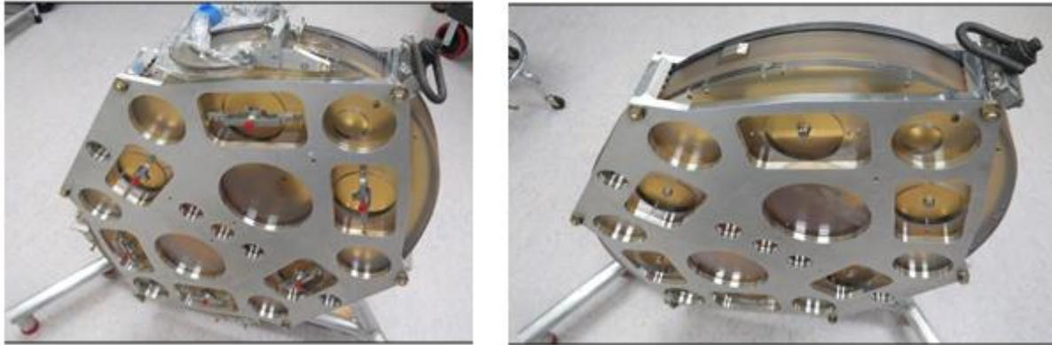
Figure 3 - Mirror at Keck in the glue jig fixture. The fixture is on a stand so that the tooling can rotate about the mirror center. This allowed positioning the three lateral pucks on edge to be individually upright for easy work access. Left image is mirror fixtured prior to bonding. Right image is after bonds sufficiently cured and with puck positioning hardware removed.
