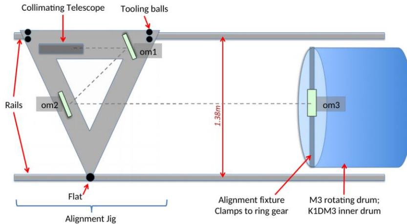
Figure 14: Schematic of Alignment Jig, Alignment Fixture and Module for alignment of module rotation axes. OM1 and OM2 redirect the beam from the collimating telescope to the module and OM3 has tip/tilt adjustments to align normal to the rotation axis
