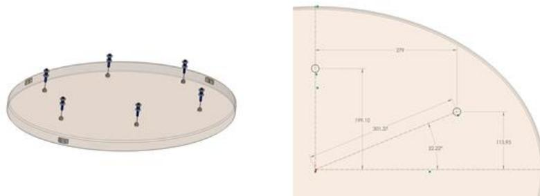
Figure 4 - The left CAD image shows the six axial support rods attached to the back of the K1DM3 mirror. The diagram on right shows the placement of two of the rods indicated by open circles. The measurements are referenced from the major and minor semi-axes of the mirror.
