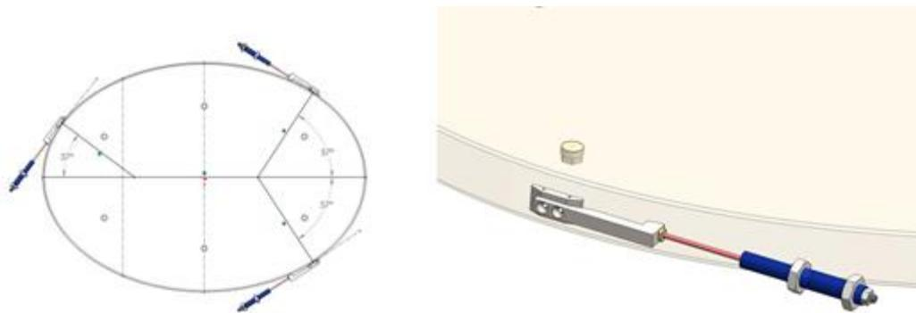
Figure 5 - Left diagram shows the placement of the three lateral supports along the outside edge of the mirror. Right image is a close-up view of one of the lateral supports screwed to a puck that is glued to the edge of the mirror.
