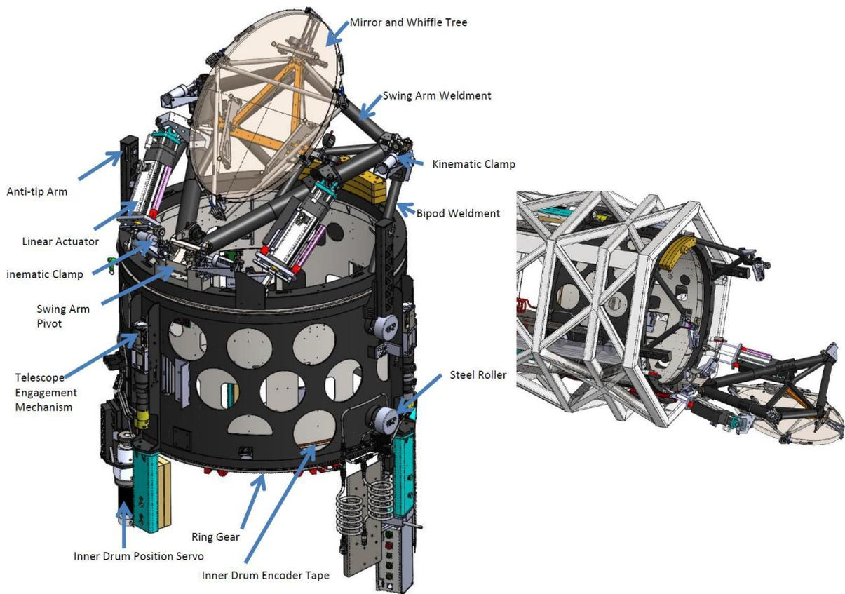
Figure 1: The Keck 1 Deployable Tertiary Mirror (K1DM3) in its deployed state (left) and in its retracted state installed on the tertiary tower (right)
