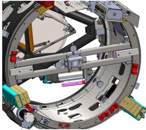
Figure 17: Ring gear attachment with OM3 on tip/tilt/translation stage
