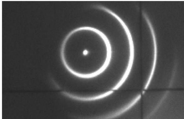
Figure 15: Autocollimation image. The rings are at radii 1,2,3 ..arcminutes. We can locate the center of the “bull’s eye” to about 0.5 pixels which is 1 arcsecond resolution.
