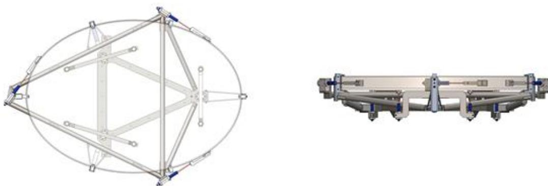
Figure 6 - Top and side views of the whiffle-tree support structure for K1DM3.
