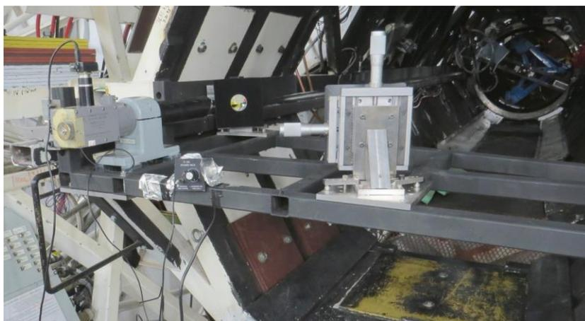
Figure 16: Alignment jig on rails of Keck-I. Autocollimation telescope with CCD camera
