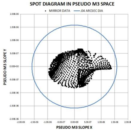
Figure 9 - Spot diagram based on results shown in Figure 9. This diagram represents where light reflected by the mirror would strike the focal plane. The image is a family of points which are calculated based on the slope error throughout the mirror. If the mirror were not deformed (perfectly flat) the image would be single point at the center.
