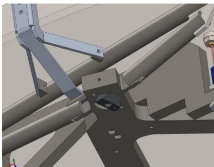
Figure 7 - At the center of the image is the kinematic coupling (canoe sphere) for attaching the mirror assembly to the swing arm assembly.
