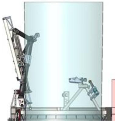
Figure 2 - M3 in retracted position and clearing the FOV to the Cassegrain instruments.
