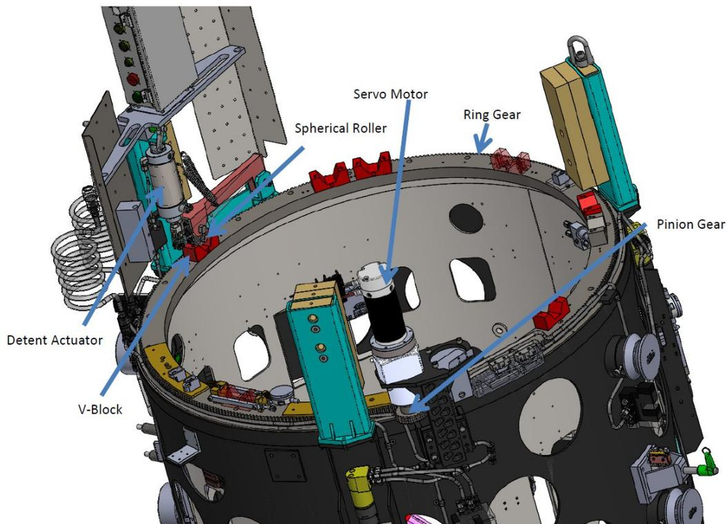
Figure 12: Azimuth/instrument positioning system, spherical roller engaging in v-block
