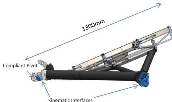
Figure 11 - Views of the mirror support swing arm, dimensions are in millimeters, canoe sphere kinematic interfaces highlighted in blue.
