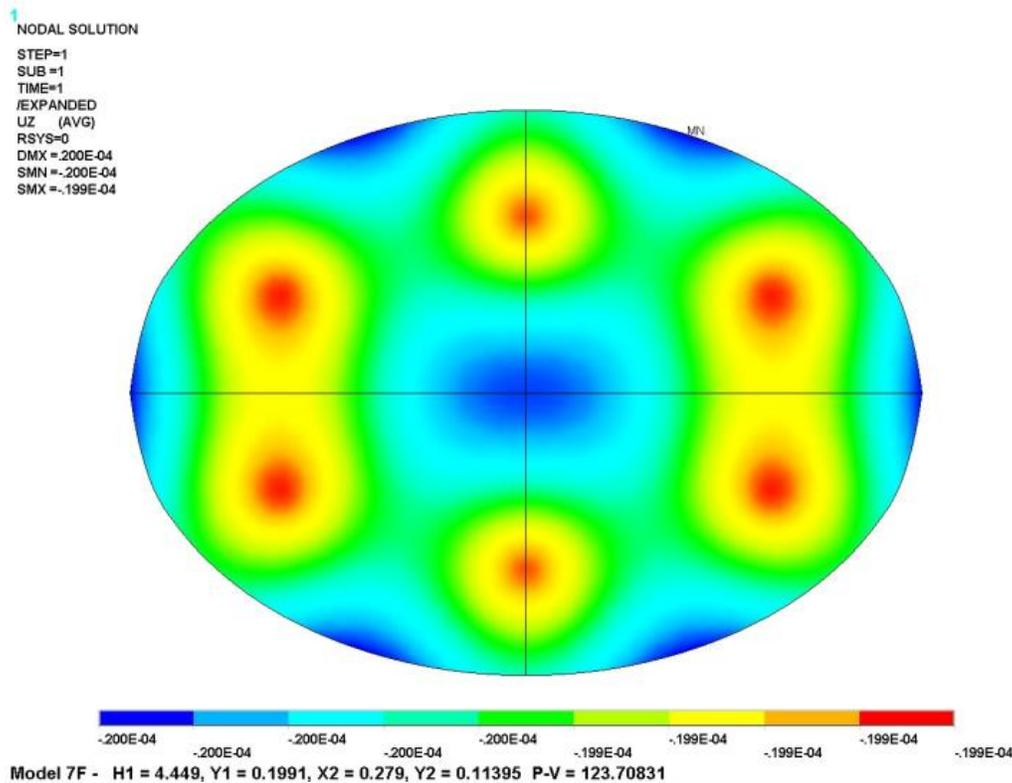
Figure 8 - Surface deformation map for the six point support system due to gravity normal to the mirror. Deflections are in meters. The contour map is for the entire mirror surface. The peak-to-valley range is 124 nm. RMS deflection of the entire surface is 39 nm.
