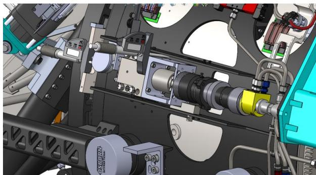
Figure 18: Defining point mechanism assembly with adjustment tooling
