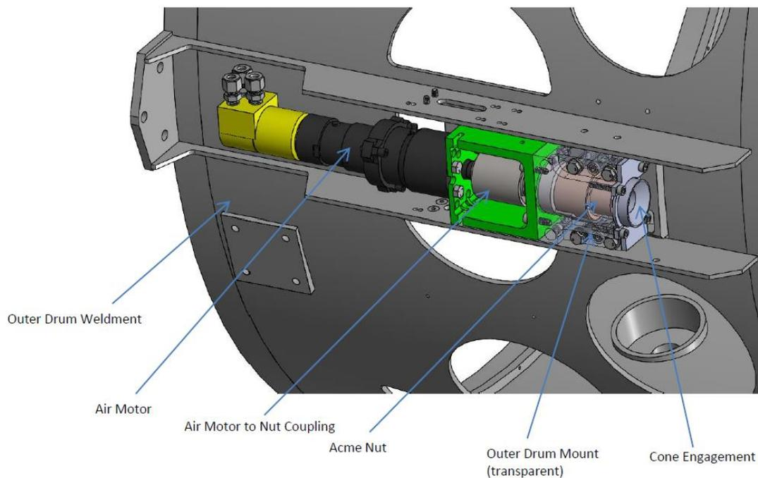
Figure 13: K1DM3 tertiary tower engagement mechanism, cone type. Outer drum mount shown as transparent to show internal parts
