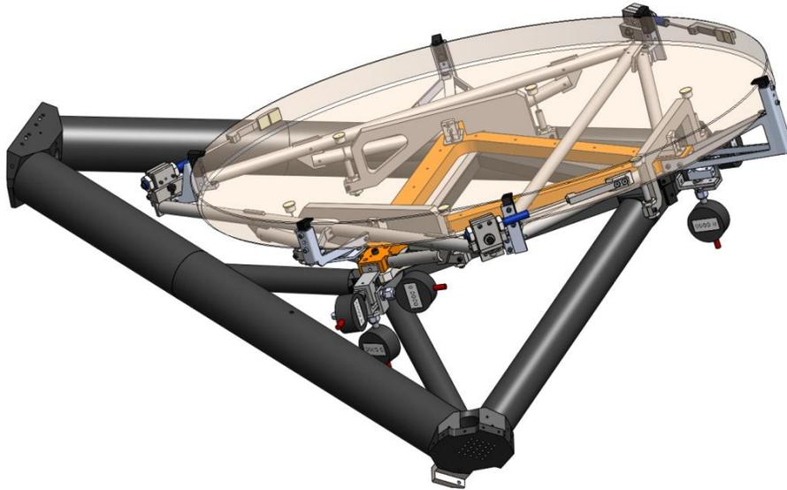
Figure 21: K1DM3 Tip/Tilt/Piston M3 Adjustment Tooling Relative to Swing-Arm
