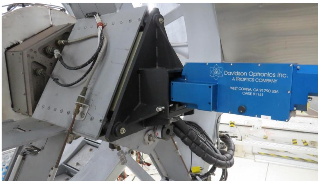
Figure 20: Automated alignment telescope mounted to Keck-I f/25 secondary, looking through the central hole in the mirror. Tested August 2017. There are tilt-tip adjustments in the mounting bracket, but the actual pointing of the alignment telescope is not critical as long as the targets can be clearly seen.
