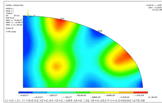
**Figure 5:** This color contour map shows the deflections of the FEA model for full gravity load perpendicular to the surface with a 12 point axial support. The support locations are indicated by the three small black dots. At these locations the vertical deflections were constrained to be zero. The peak to valley deflection is about 20 nm.
