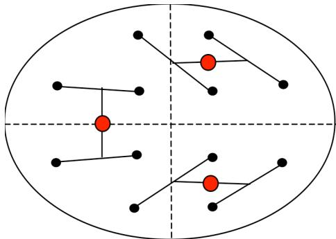
**Figure 4:** This cartoon shows approximately the locations of a 12 point axial support system and how they might be combined with whiffletrees to three location points that would form the attachment locations to the outside world.
