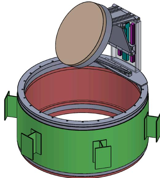
**Figure 6:** The K1DM3 “tub” which serves as the mount for the deployable tertiary. Aside from the custom bearing, all parts shown are standard, off-the-shelf items.
