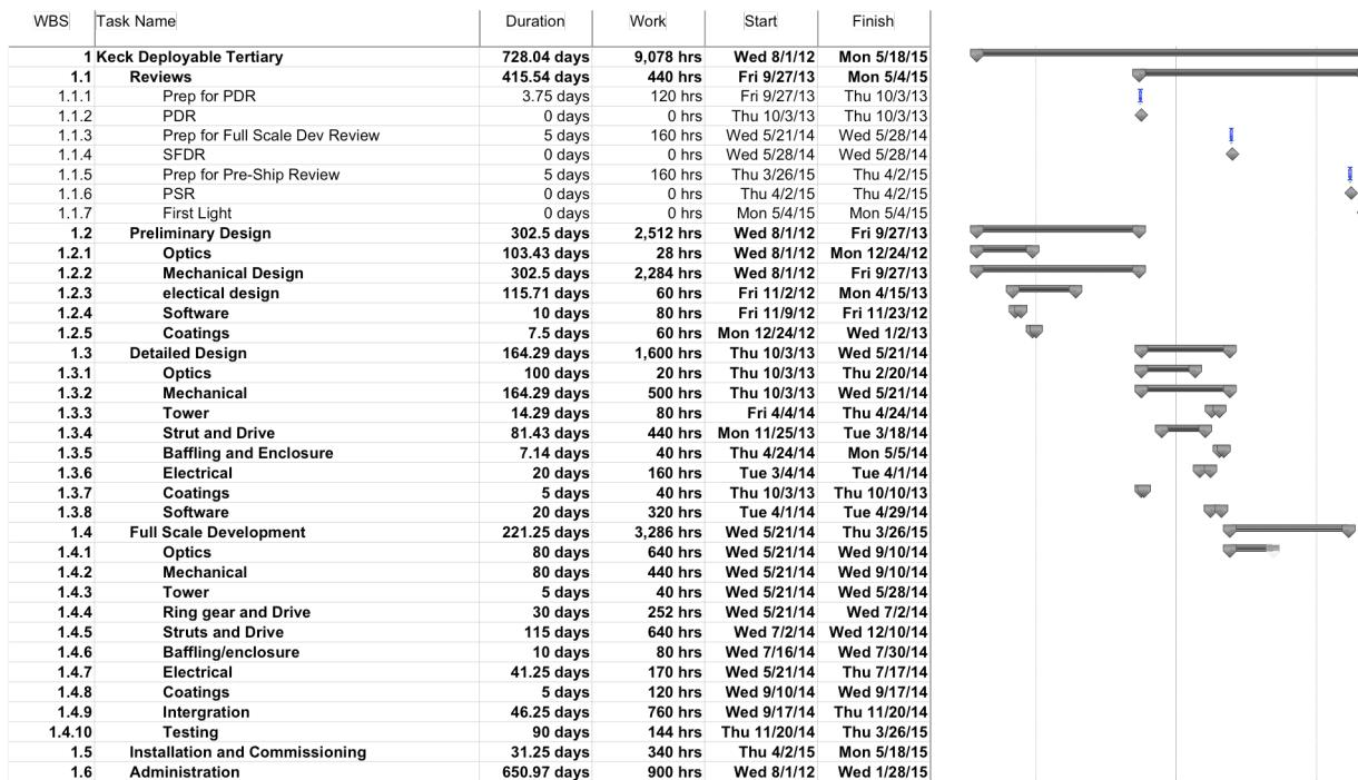
**Figure 10:** K1 Deployable Tertiary (K1DM3) project Gantt chart and WBS.
