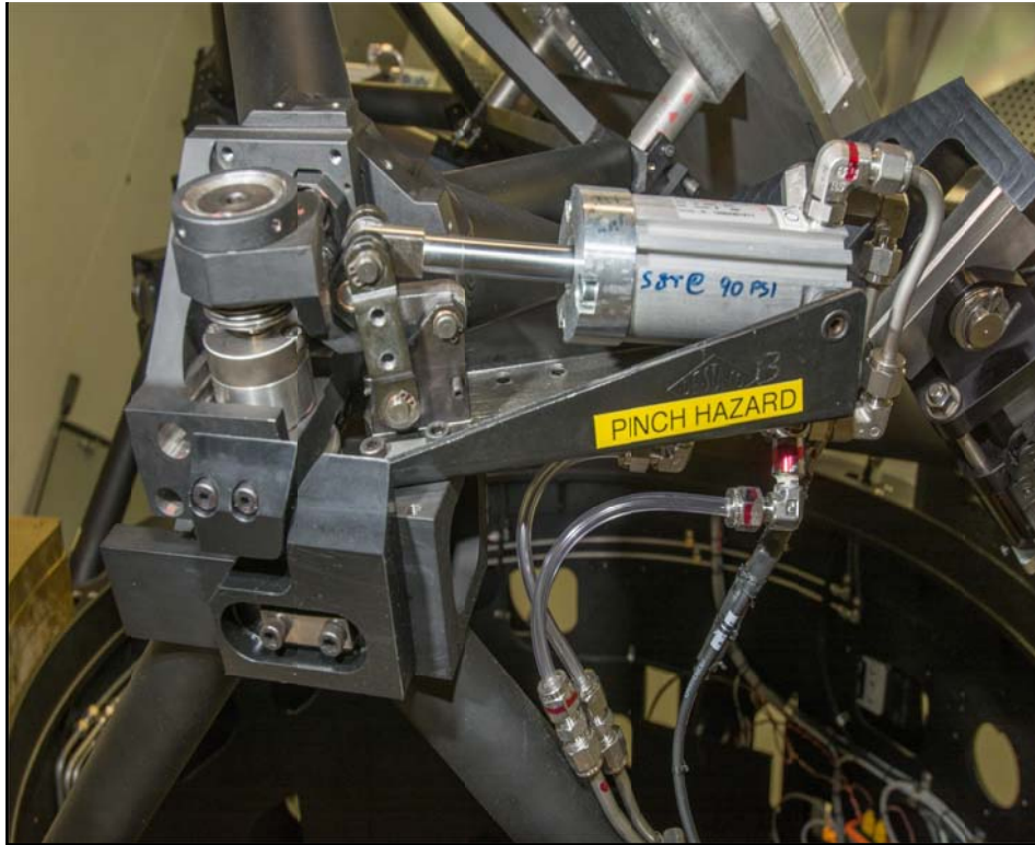
Figure 4 - Clamp/Air Cylinder at one of the two bipod locations
