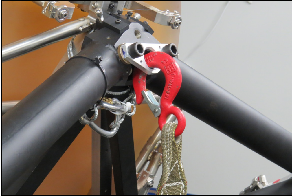
Figure 1 - Lifting eye plate with come-along attached. Fasteners are M12 fine thread SHCS
