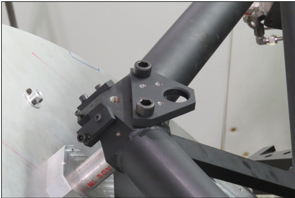
Figure 2 - Redesigned lifting eye for easier connection with hook.
