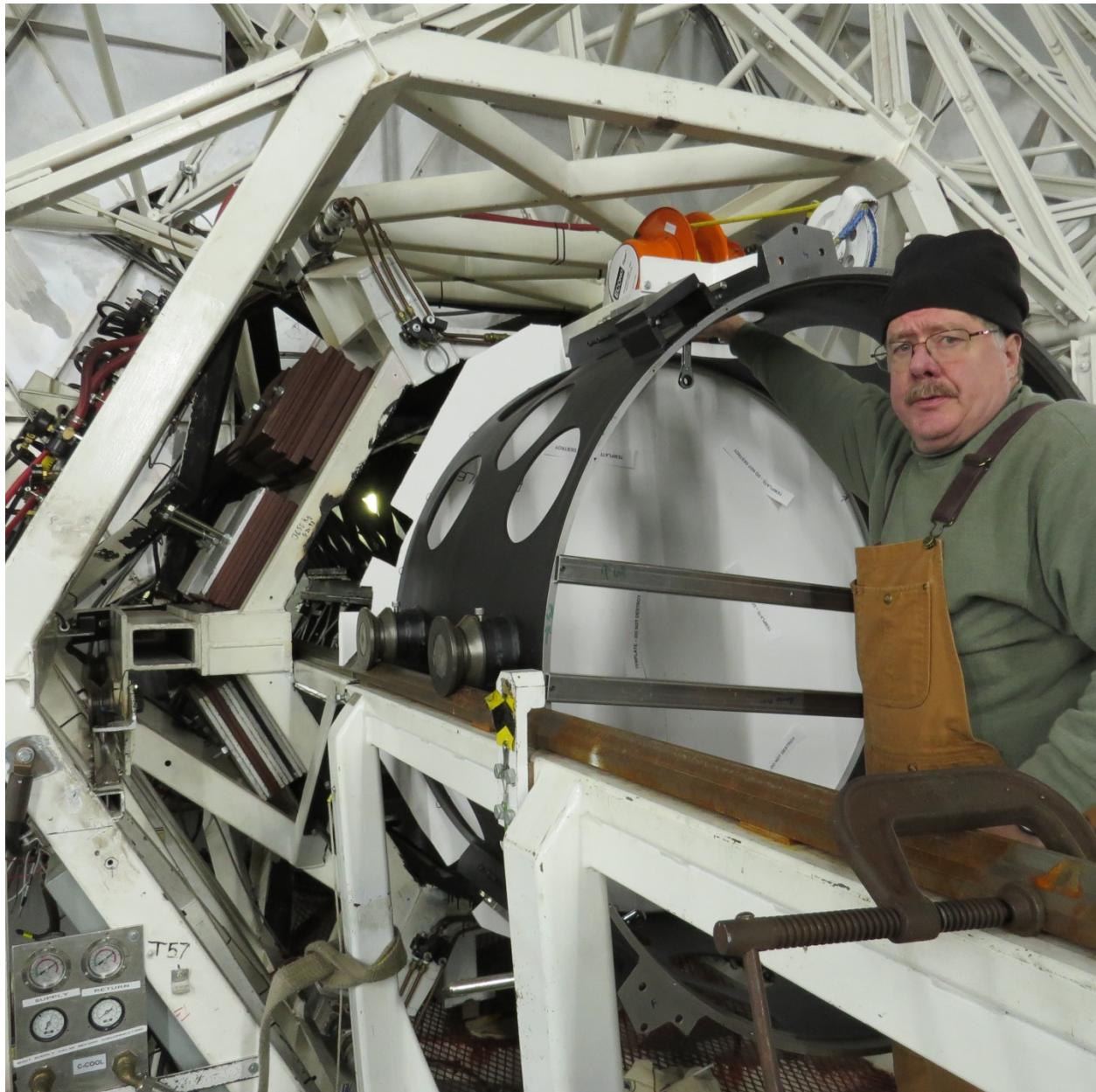
Figure 2 – Jim Ward commencing to push foam core through the tertiary tower, another person is further up the tertiary tower to cut away interfering material
