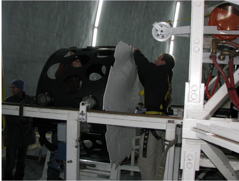
Fig. 10.— ODF fitted with the foam core.
