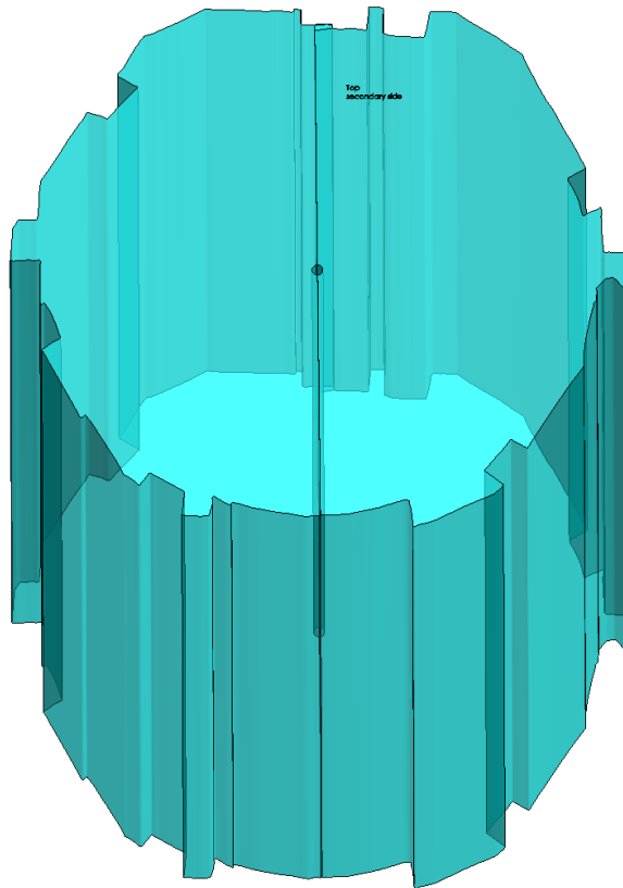
Fig. 11.— CAD model of the foam core.
