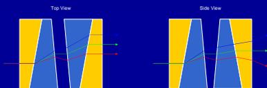
Schematic of crossed-Amici ADC, showing the null configuration (left), and maximum correction (right)
