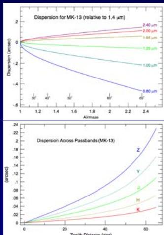
Differential atmospheric refraction relative to 1.4  $\mu\text{m}$  (top), and the edge-to-edge differences across individual passbands (bottom) for the Mauna Kea site chosen for TMT.
