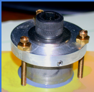
Gluing jig used to control test sample bond thickness.
