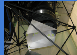
Bonded cross-dispersing prism mounted within the instrument structure.
