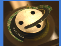
Bonded puck showing epoxy fillet and its removal.
