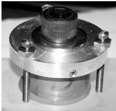
Figure 1 - Gluing fixture used to prepare test samples. Note the three outboard screws used to set adhesive gap.
