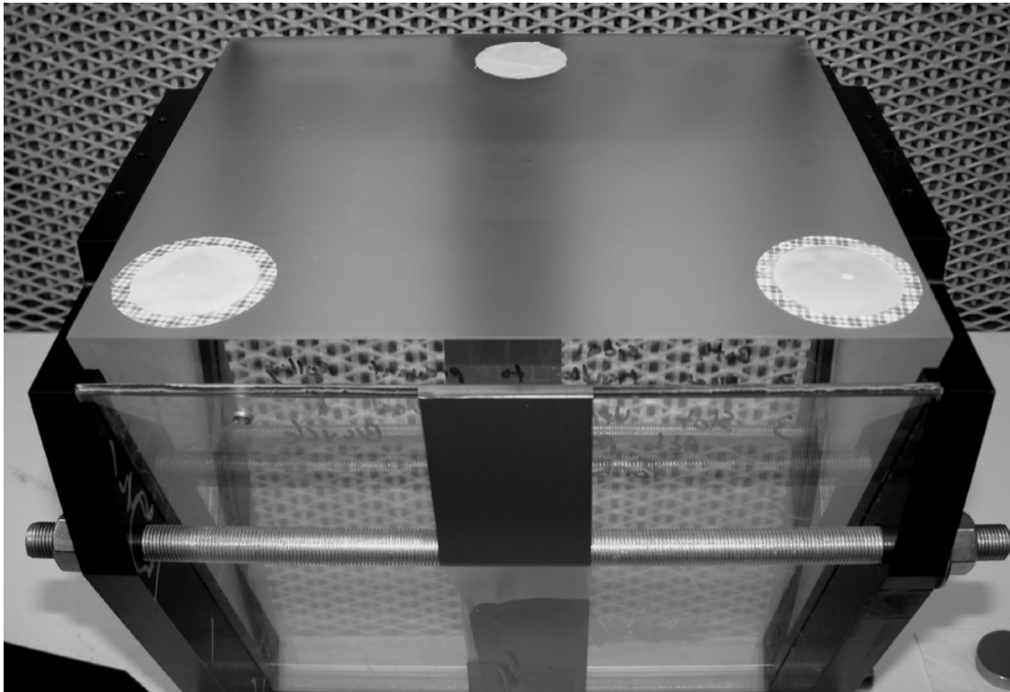
Figure 5 – Prism in its handling fixture showing primed bonding areas prior to sanding. Primer masking ring has been removed from the rearmost area.
