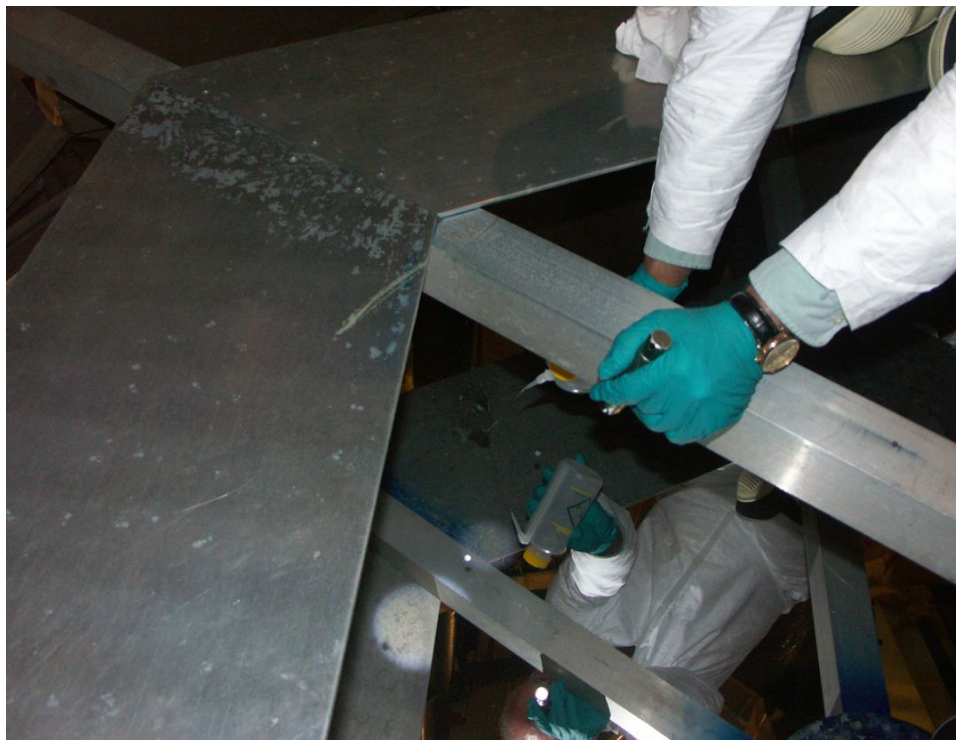
Hazy surface in field area of primary mirror
