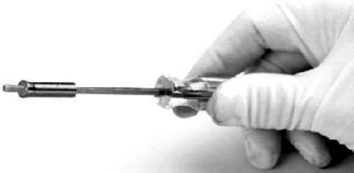
Figure 5-3. Socket-head screw correctly retained by the sleeve on the end of the Allen driver
