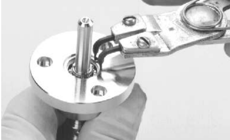
Figure 5-19. Removing the retaining ring that secures the outer crucible drive bearing in the bearing housing
