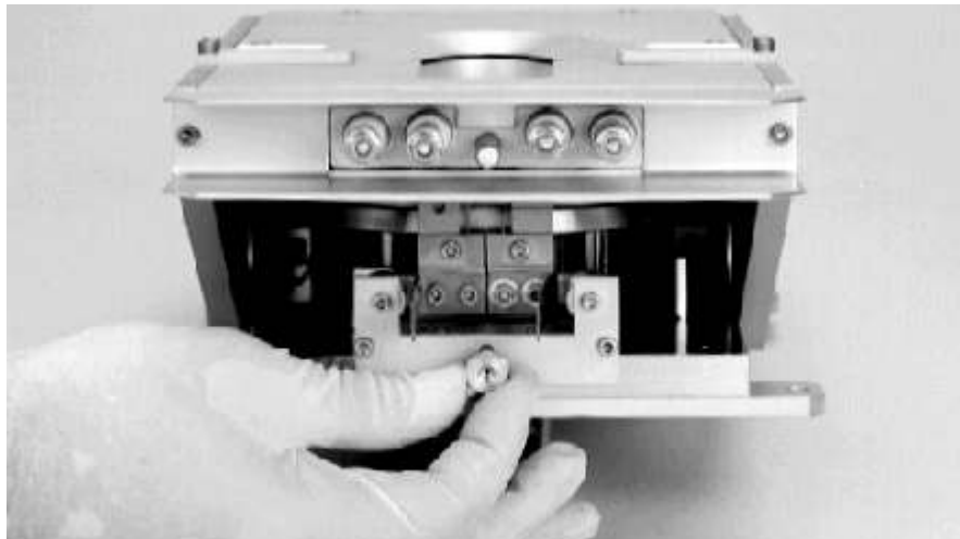
Figure 5-6. Removing the emitter assembly
