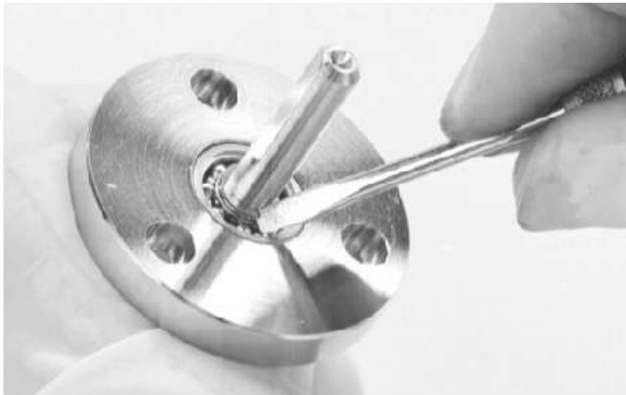
Figure 5-20. Removing the retaining ring that retains the drive shaft
