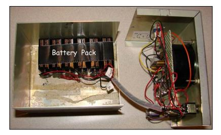
Turn on the unit with the sensor attached and sitting on the witness mirror. Place the sensor filter to Blue and using the knob labeled Lamp adjust the meter needle to 10. If the needle will not make it up to 10 replace the batteries. If while using the meter it continually drops while zeroing the meter, replace the batteries. Recycle the spent batteries properly.
