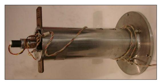
This is the sensor unit that is placed on the optic for testing. It has three small nylon feet that rest on the optic surface. These plastic feet help to reduce damage to the coating and optic. When placing the sensor use straight up and down motions only. Never slide the sensor on the optic surface as this would result in significant damage to the optic.
