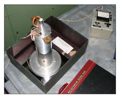
**Introduction:** This reflectometer is a "Lick built" instrument built many years ago and is fairly primitive. It is still good at comparing the coating to be tested against the quality of the witness mirror and is very easy to use.
