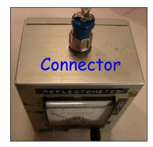
The sensor unit plugs into the top of the electronics box and the plug retainer is then locked into place to insure a good connection and the plug won't fall out and drag across the optic being tested.
