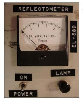
The instrument is quite simple to use. The electronics package has the power switch, lamp adjustment knob and meter.
