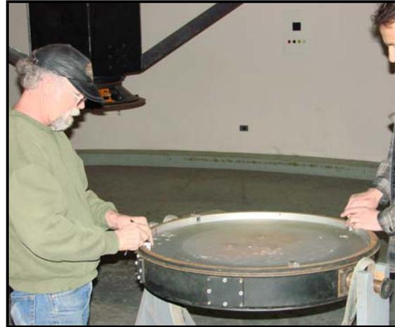
Remove the bolts holding the cell to the secondary frame and move the secondary frame out of the way.
