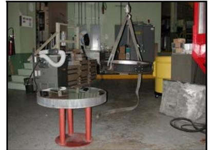
Set the mirror on the stool and remove the four safety clips and remove the cell.
