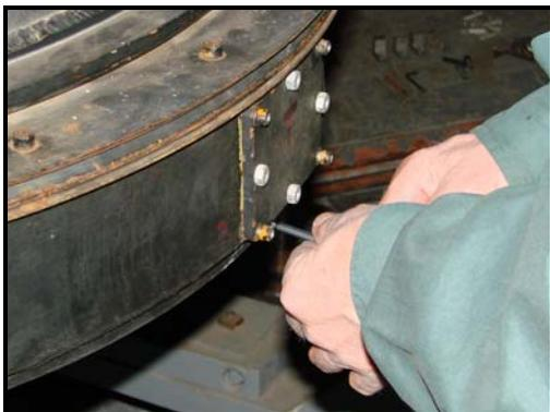
Remove the four bolts on the corners. Do not touch the setscrews with locking nuts. They are preset for positioning the glass properly.
