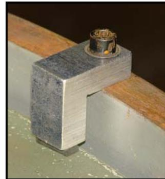
Four safety clips must be installed to hold the mirror when to enable flipping the mirror over. There should be foam on each clip surface that touches the glass for padding.
