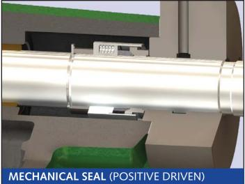
These are positive driven seals with a PTFE wedge, for use where corrosive and/or viscous liquids are being processed. Wedge construction of the secondary sealing element virtually eliminates leakage. These seals have a temperature limit of 450°F (232°C). Special fitting is available for higher temperature applications.
