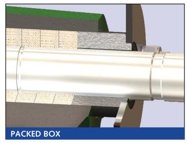
The packed box seal is suited for general purpose applications. The standard packing has a temperature limit of 250°F (121°C), with special fitting available for higher temperature applications. The gland should be adjusted to allow slight seepage.
