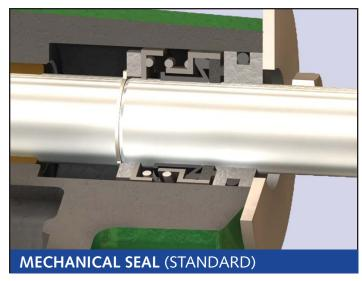
Mechanical seals are for those applications where product leakage is unacceptable. The mechanical seal uses less power than the packed box and, under proper conditions, has a longer service life. It does not require adjustment. Our standard mechanical seal is an elastomeric bellows type seal, with a temperature limit of 212°F (100°C). Special fitting is available for higher temperature applications.
