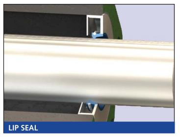
The lip seal is suitable for low pressure sealing of lubricating fluids. The standard seal has a temperature limit of 212°F (100°C). Special fitting is available for higher temperature applications. Available in CW rotation only and 100 psi maximum discharge.
