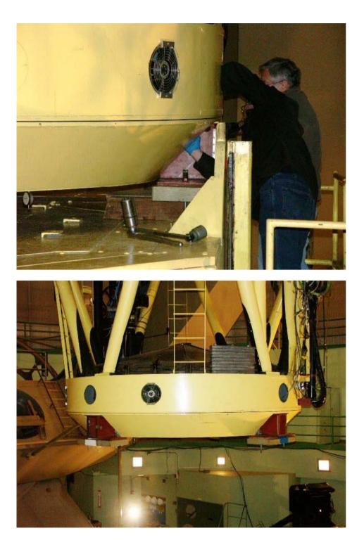
Then the "hub" of instruments was hoisted over to the platform and re-attached to the telescope.
