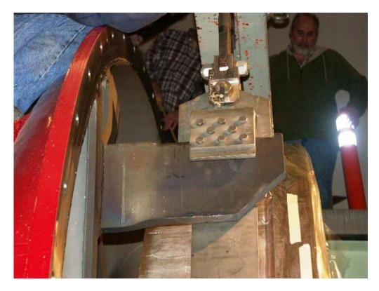
The mirror was anchored from moving inside the tank by a custom connection between the "earthquake clamp" on the mirror at the top.
