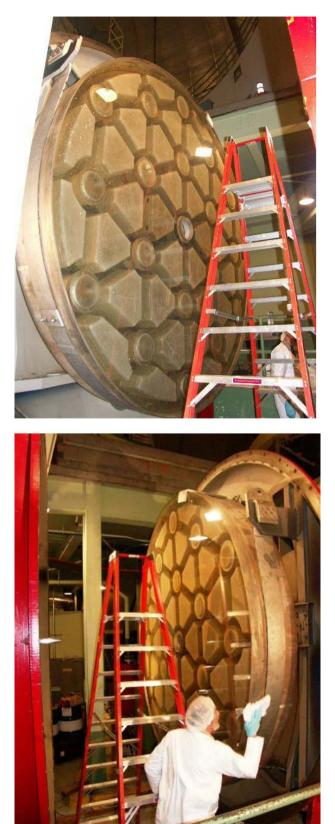
Then it was given a final wipe with 2-propanol soaking cloth towels that had been repeatedly washed to remove lint. A second, dry towel was used to wipe up the propanol before it had a chance to dry.
