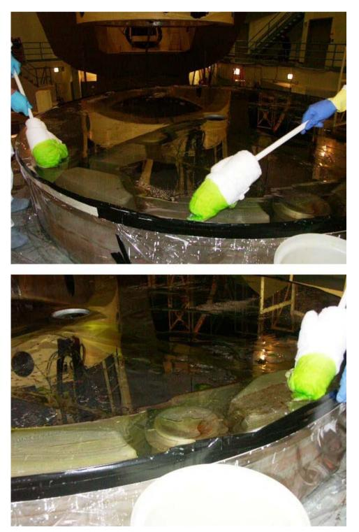
When it was all stripped we rinsed the Green River down the drain in the central hole. A second hose might have made it easier to "herd" the fluid down the drain.
