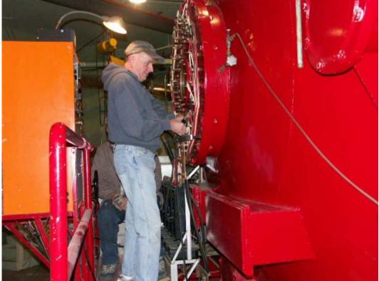
The outer ring was arranged in five sections, each with its own pre-wired source. The filaments of the outer ring were arranged so that each of the five sections had filaments in all the sections of the circumference. Darrell operated them.
