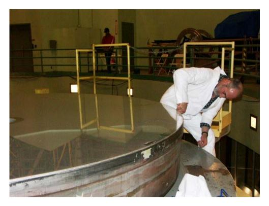
We then used a layer of masking tape and a layer of double-sided tape to attach a 3' or 4' wide skirt of vinyl to the mirror, draping it down to protect the painted surfaces and the people working below from the fluids we were preparing to use. We had to put the vinyl on in several sections, and we were careful to overlap the sections with more vinyl and to seal the joints with duct tape.
