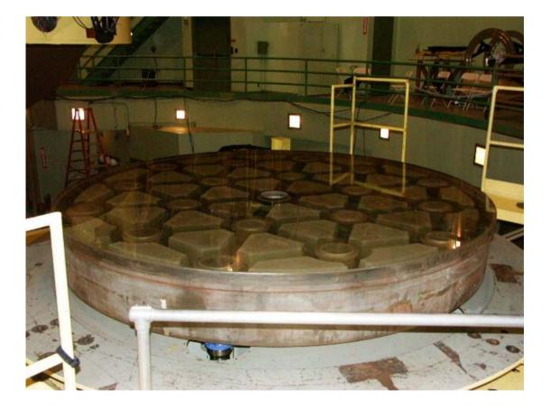
The last step for the night was to cover the mirror with cellophane, which came on a roll in a 4' wooden box. We taped it to the edge of the mirror on one side and unrolled it without dragging it on the surface, then taped it down on the other side. This is another area where we suggest improvement...perhaps a giant shower cap made of sail-cloth or some other light material. Something in the center hole would keep it from touching the surface of the mirror.
