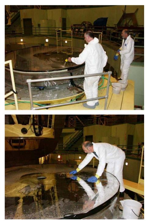
After washing we dried just the same four locations for the reflectometer. We repeated the measurements and found that just washing it increased the reflectivity from 73% to 83%. Since we were going to strip it we didn't worry about the water drying in spots.
