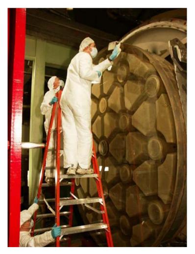
Finally, dry nitrogen from an anti-static gun was used to blow off the surface.
