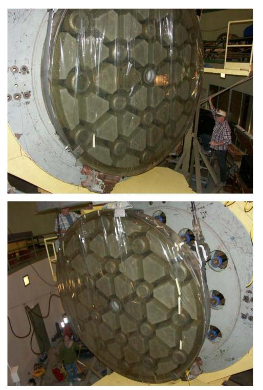
Using manned ropes to keep the mirror from swinging, the crane brought the mirror over the coating chamber.
