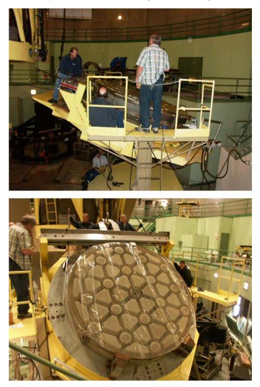
The crane was raised to just lift the mirror off the edge-arcs, and the platform was driven south to separate it from the mirror.
