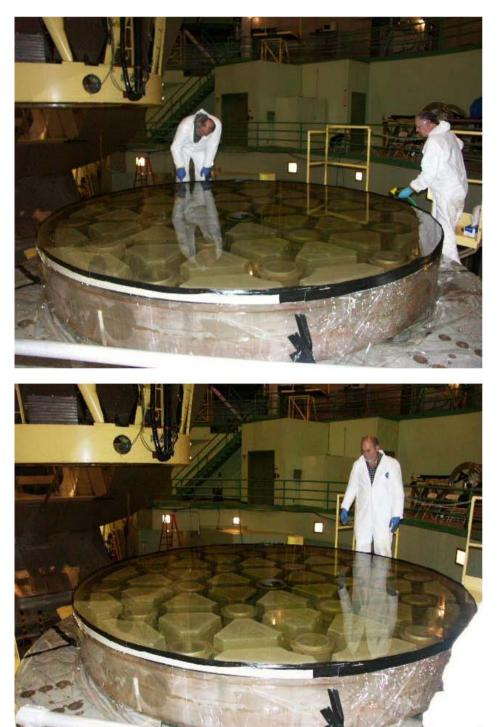
We then went right into the cleaning process by swabbing the surface with KOH / H2O using fresh Q-Tips. Bill then sprinkled copious amounts of CaCO3 (calcium carbonate) on the wet surface and we used Kaydrys dipped in the KOH / H2O solution to make "toothpaste" of the CaCO3. We rubbed the surface all over and then rinsed it down the center hole. Again, a second hose might have made it easier to "herd" the fluid down the drain.
