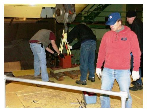
Later the other three were put on the platform. It was noted that the alignment marks for the weights had been painted over, so there was some pushing and pulling on the massive weights that was required to get them in to position. Next time the mirror comes out the positions of the weights should be re-marked before they are taken off. This will make replacing them much easier.
