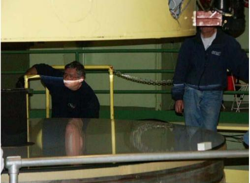
We next removed the old foil, tape and cardboard from around the circumference of the mirror, cleaning off the tape residue with acetone.
