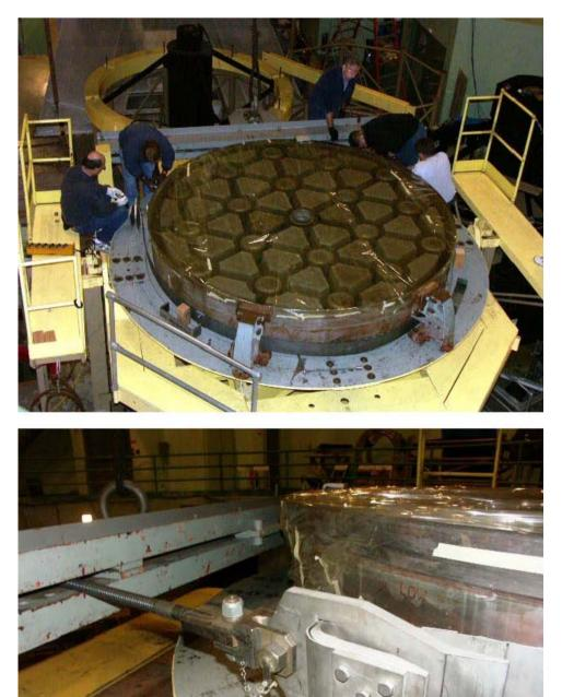
Here is a close-up of the top of the jackscrews, showing the hand-grips for tightening or loosening the bellyband.
