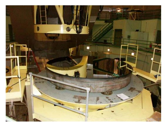
Once there, we put a new skirt of foil around it. We changed the procedure slightly in that we used black duct tape in place of the beige masking tape in direct contact with the mirror. This was because it had been hard to get the old tape off and it was thought that the fiber backing of the duct tape would make it come off easier (we anticipate having to remove more tape residue with acetone).
